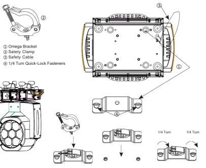
Regardless of the rigging option you choose for your BLUR 715, always be sure to secure your fixture with a safety cable. The fixture provides a built-in rigging point for a safety cable on the hanging bracket as illustrated above. Be sure to only use the designated rigging point for the safety cable and never secure a safety cable to a carrying handle.
